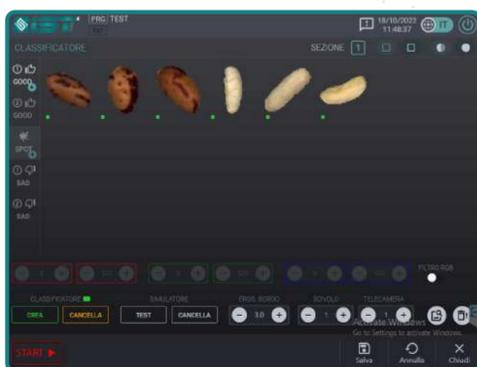
An **internally developed** software intended to allow the operator to manage programs in a fully autonomous way. A **self-learning** system can be used to set up a program within just a few minutes, which automatically captures images of compliant products and all defects to be discarded.
